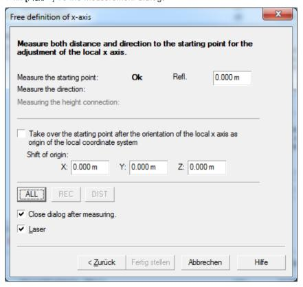
Measure 2 points on the same wall. The two points should be at least 1m apart, they should also be measured at approximately the same height.
