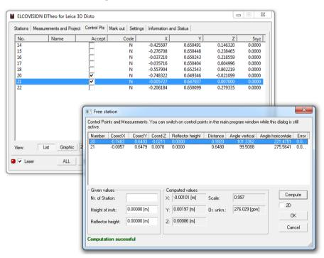
For free stationing there must be at least two known stationing points. The stationing points can be selected from the coordinate list or the corresponding graphical overview. The points of the coordinate list either originate from the measurements already taken or have been added to the project by means of an imported coordinate file.
