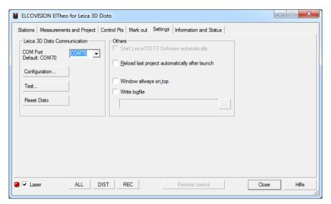
If the Leica Windows software for the 3D Disto has been installed without any changes, no further settings are necessary. If necessary, the COM port must be reset.
