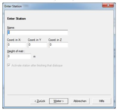
If you later need the position as a check point or connection point for a further position, the instrument height (distance floor - tilting axis of the 3D Disto must be entered!
