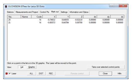
This page is very easy to use for staking out: On the "Control Points" page, first select the points you want to mark out and then switch to this page. By clicking on [Take over selected control points] these previously selected points are transferred to the list.
