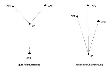
By using only 2 connection points it is not possible to check the determined position!
