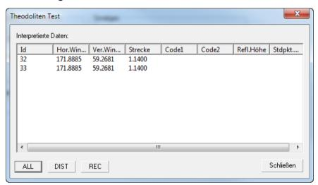
In this sub-dialogue of the settings can be checked whether a data transmission between the computer and 3D Disto takes place. In the figure above is an example of a correct data transmission is seen. EITheo automatically converts the links in the geodetic system measured values for values in a mathematical system of law.
