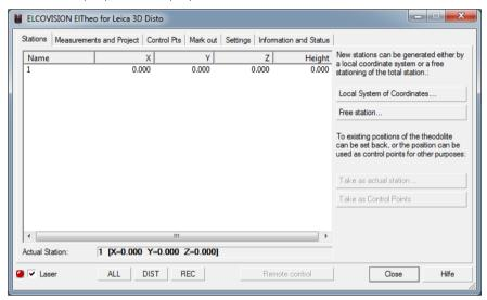
On this dialogue page new points of view can be created, or the Disto can be repositioned to a previously existing point of view. With free stationing, the 3D Disto can be set up and reoriented at any point.
