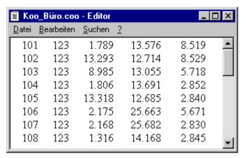
The point number can have alphanumeric designations. Very important is the presence of the point code. The code determines whether the point is interpreted as a full or partial pass point or simply as a new point.
