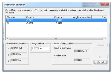
To complete the orientation, the direction angles (horizontal angles) to the individual connection points must be measured.
