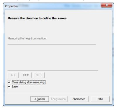
Here the direction (horizontal direction) in which the X-axis of the new local system is to be placed is determined. This is also called orientation of the coordinate system. The measurement can be started directly on the 3D Disto with the small remote control, or with the Leica 3D Disto Windows software, or by clicking the [REC] button in the dialog.
